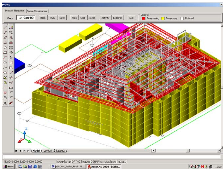
Figure 3.10: 4D Visualisation for Constructing Centuria Building (Construction Situation of Purlins of the Roof on 14/01/2000)
