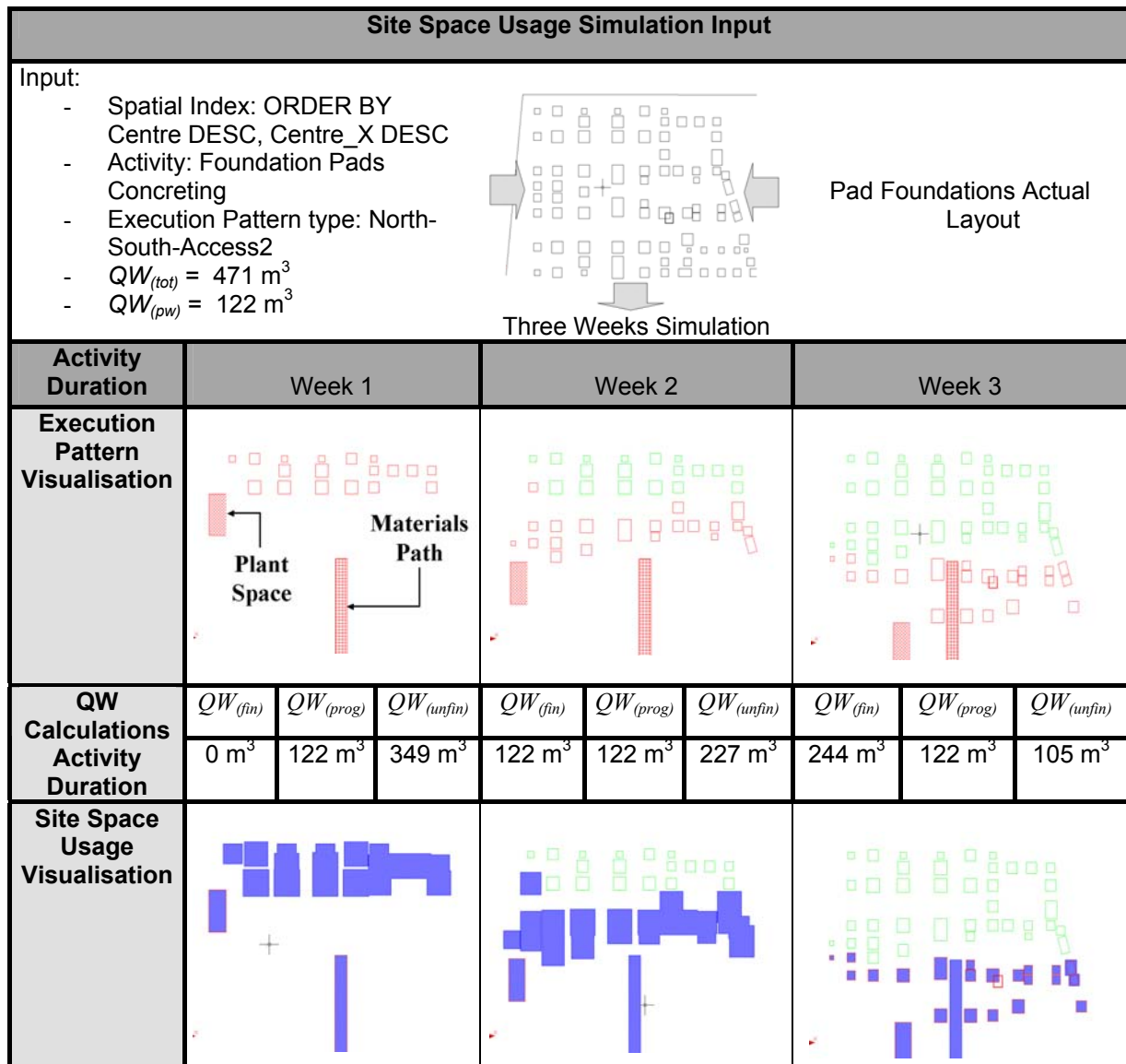
Figure 3: Visualisations of Quantity of Works combined with an activity execution pattern
