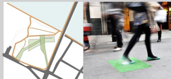
HARVESTING KINETIC ENERGY FROM PEOPLE MOVEMENT - PAVEGEN SYSTEMS
